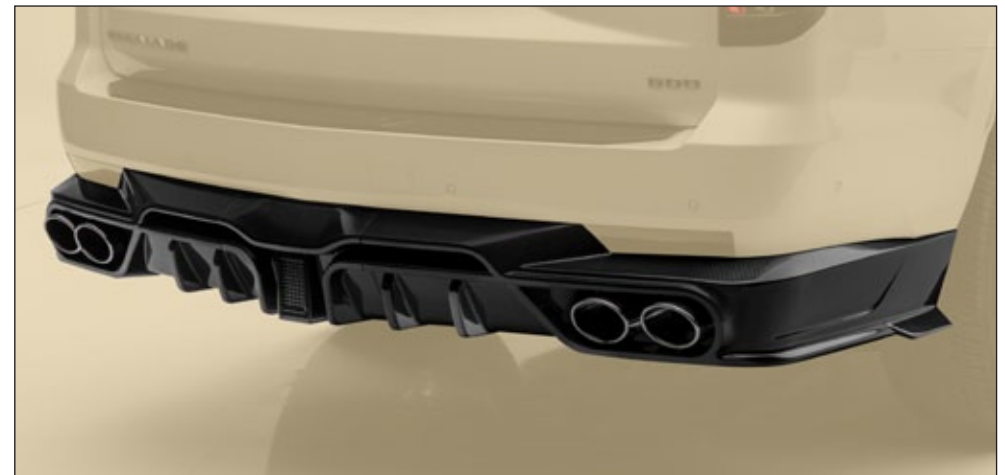
Rear diffuser with race brake light
