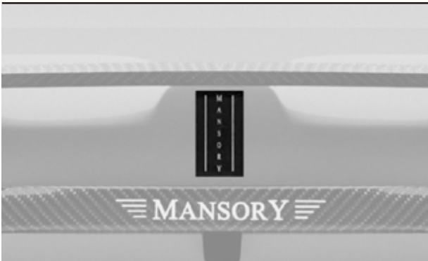
Mansory emblem for tailgate with engraved logo RCS 730 991 visible carbon fibre primed without clear coat
