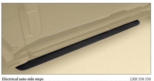
Electrical auto side steps 2 parts set - left & right, additional parts with integrated LEDs 200 kg load capacity (each side)
