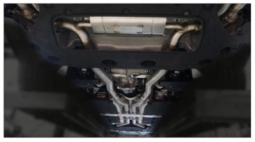
Sport Exhaust Muffler for MANSORY Rear diffuser End muffler ① Only for export!
