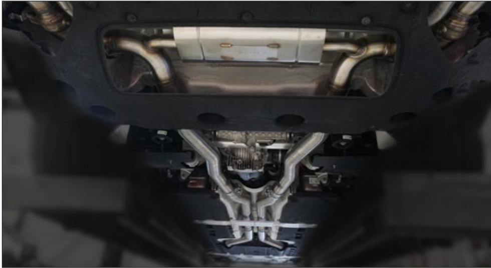
Sport Exhaust Muffler with down pipe for MANSORY Rear diffuser LRD 222 229 with alluminium double exhaust blinds, Exhaust remote control with CAT 200 cell, End muffler ⓘ Only for export! ✘ Compatible only with MANSORY Rear diffuser
