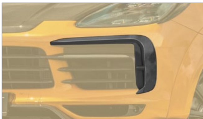
Front bumper covers add-on (Cayenne V6) ..... PCN 152 851 2 parts set - left & right, visible carbon fibre without clear coat compatible only with: Cayenne, Cayenne S, Cayenne GTS ⓘ not compatible with Cayenne TURBO
