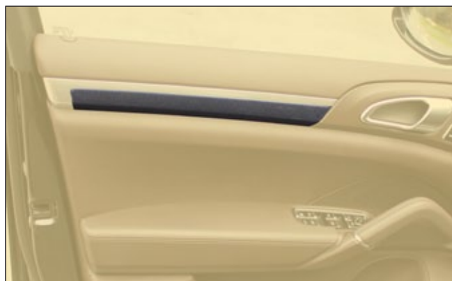
Door Panels PNC 405 00 4 parts set - front/rear, left/right, available with carbon fibre or wood veneer. ⚠ modification only, OE-part required
