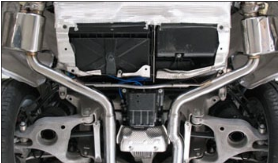
Sport exhaust with throttle system for serial rear bumper ..... PNC 300 02 Sport muffler with throttle left & right Remote control, Extension tail pipes and assembling parts.
