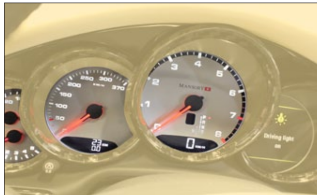
Speedometer display PNC 414 00 new designed Instrument dials, inclusive speedometer upgrade, custom colour On request ⚠ modification only, OE-part required
