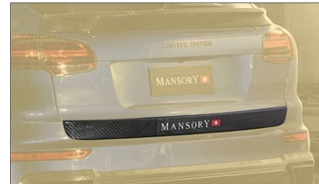
Rear hatch panel ..... PNC 802 741 with MANSORY logo visible carbon fibre primed without clear coat
