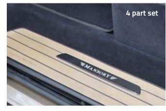
Sill plates with Illuminated MANSORY logo 448 385 351 4 parts set, visible carbon fibre primed without clear coat with illuminated MANSORY logo Sill plates with MANSORY logo 448 385 355 4 parts set, visible carbon fibre primed without clear coat with MANSORY logo
