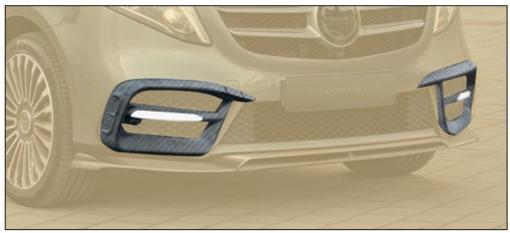
Air intakes with LED day running lights visible carbon visible carbon fibre primed without clear coat
