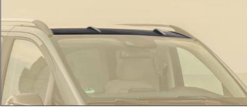
Roof panel 448 110 158 visible carbon fibre primed without clear coat
