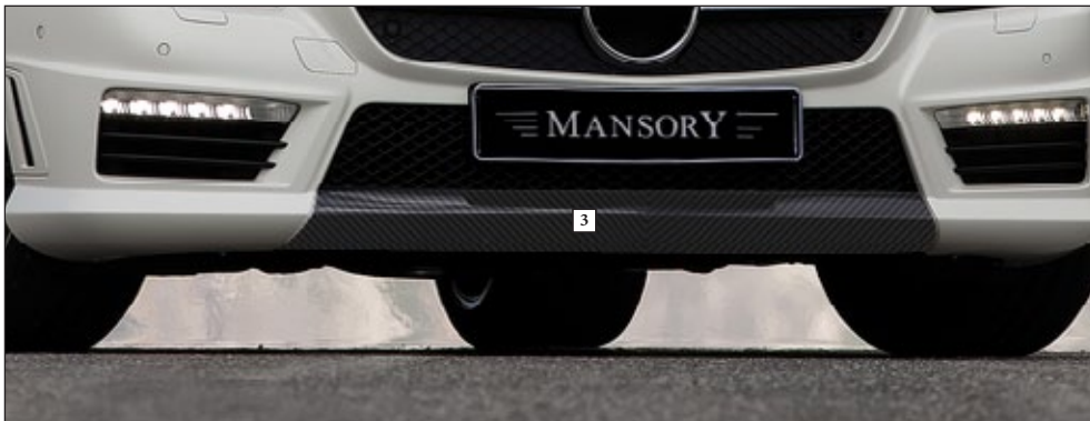
3. Front splitter cover AMG ① Only for AMG 6.3 - A172.102.851 visible carbon fibre primed without clear coat
