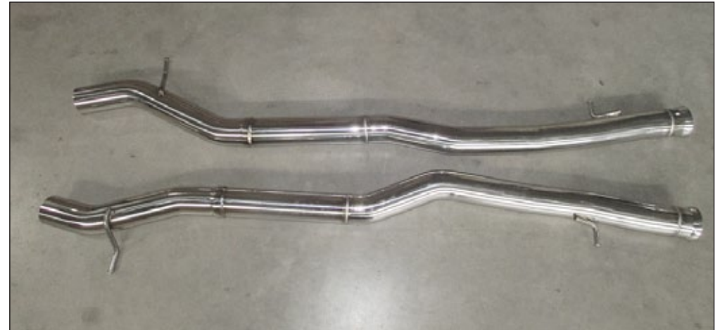
Exhaust middle pipes
