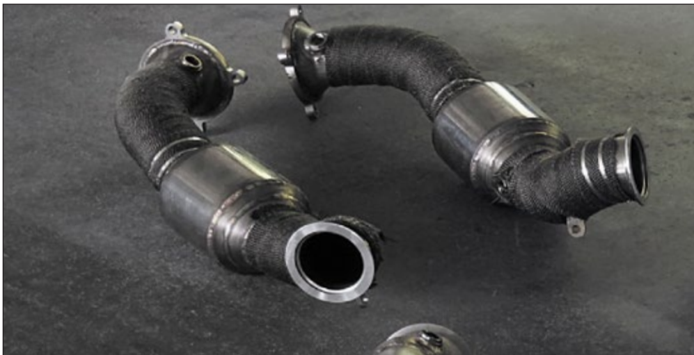
Down pipes with cat 200 cell
