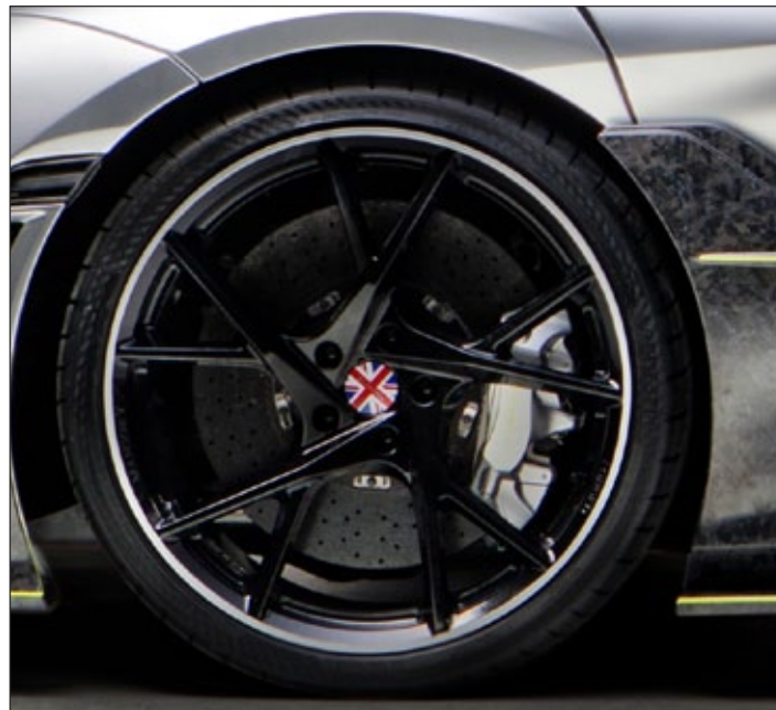
Yavin ultra-light forged wheels FA: 9.5 x 20 inch YN5 20 95 34 112 R RA: 11.0 x 21 inch YN5 21 11 14 112 R
