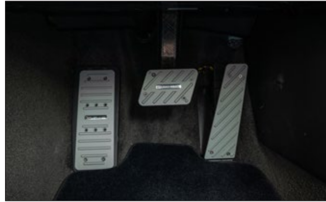
Sport pedals BX7 367 127 3 parts, acceleration, brake, foot rest
